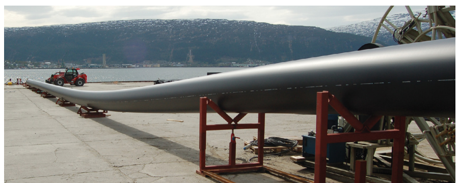
Fig. 6 – Extrusion of an 800 mm pipe
